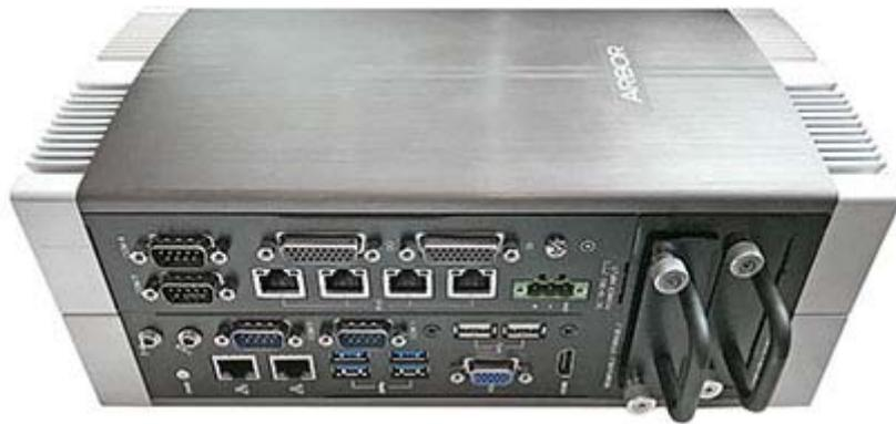
The image below to the right shows how two heat spreader housing modules are combined to create the ARES-1970-E version. This increases size to 10.71 x 5.55 x 4.41 inches, and weight from 3.7 to 8.2 pounds. It also means the unit can be used standing up or sitting on its side (in addition to, of course, wall-mount or DIN-rail mount).
