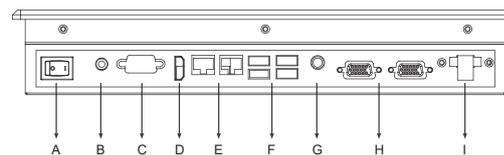
A: 电源开关 B: Audio C: VGA D:HDMI
