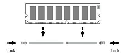
3. Fully plug the memory module until it gets auto-locked in place.
