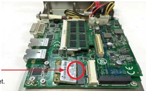
Align the notch on the Wi-Fi module with the notch in the mini-card socket.
