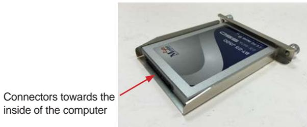
4. Carefully turn the tray over and fasten the 4 screws to secure the SSD or HDD to the tray.
