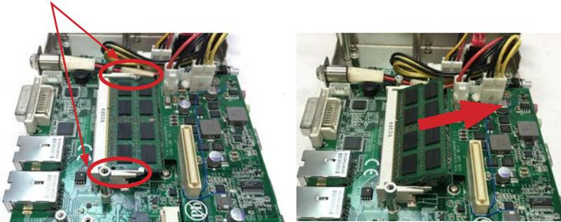
3. Confront the memory module's edge connector with the SO-DIMM slot connector. Align the memory module's key notch at the break on the SO-DIMM slot connector. By a slanted angle, fully plug the memory module until it cannot be plugged any more.
