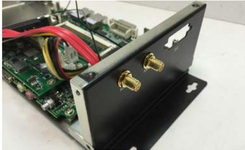
11. Prepare the external antenna. Screw and tightly fasten the antenna to the Wi-Fi connector(s). Then swivel the antenna to an angle of best signals.
