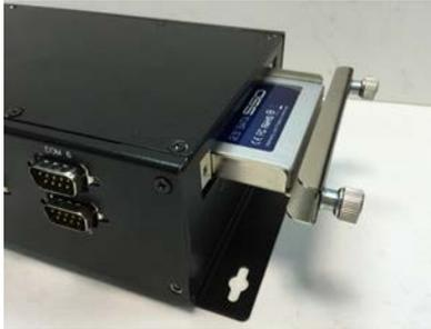
6. Fasten the 2 thumb screws of the storage tray.
