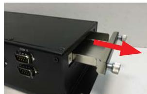
Then remove the 2 screws as shown in the image below so that you can remove the tray from the main board later.
