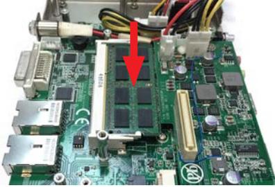
5. To reassembly the computer after the memory module installation, repeat the steps in [4.1. Disassemble the Computer](#) on page [56](#) in reverse order.
