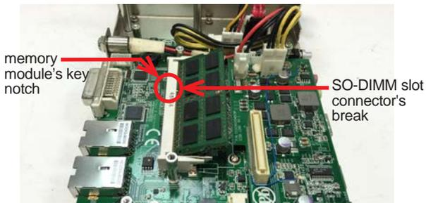
Align the memory module's key notch at the SO-DIMM slot connector's break.
