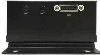
6. Remove the screw that fastens the front panel to the top board and then remove the front panel.
