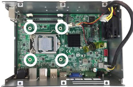
2. Tighten the four spring-loaded screws by partially tightening one pair of diagonally opposite screws and then tightening the remaining pair.
