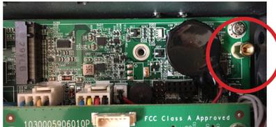
3. Insert the M.2 module into the socket by aligning the notch on the module with the small slot on the M.2 socket.
