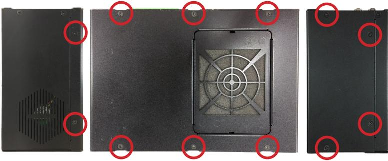
2. Then lift the L shape chassis away from the from the assembly.
