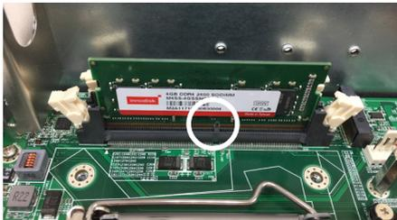
3. Press it fully into the socket until the latches lock in place.
