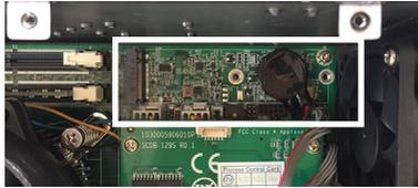
2. Insert the standard standoff into the main board.
