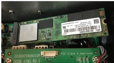
4. Insert and fasten the screw into the standoff.
