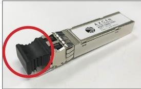
**Note:** Do not remove the rubber safety cap unless you want to install the transceiver. The rubber safety cap keep the port clean and prevents accidental exposure to laser light.
