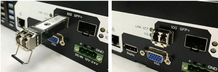
3. Then you can connect the ARES-1973C-48C8 to your network device via a fiber-optic cable.
