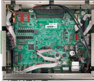
8. Locate the MBKEY slot and insert the relative communication module then fasten the screw.
