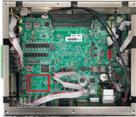
3. Prepare the Wi-Fi module kit. The module is a **M.2 E-Key** socket form factor, with two MHF connectors, one is “MAIN”, and the other is “AUX”.
