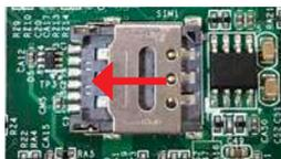
4. Insert the SIM card into the card holder as shown below.
