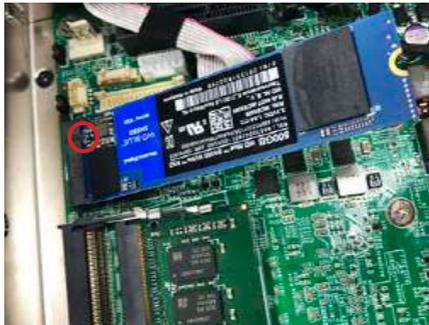
3. Insert and fasten the screw into the standoff.
