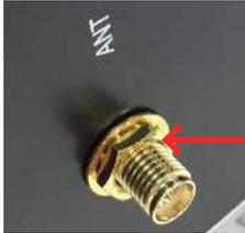
Mount the washer and the nut to the SMA connector. Tighten the nut.
