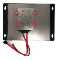
2. Slide the 2.5" HDD or SSD storage device into the drive bay and ensure it connects to the SATA connector.
