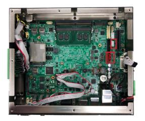
5. Secure the drive bay back to the bottom side chassis by fastening the 4 screws you removed in Step 1.
