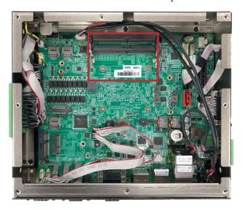
2. Align the notch on the memory module with the key in the module socket.
