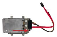
3. Using 4 screws coming with the storage device kit, fix the storage device in place.
