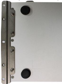
3. Use the other screw holes and cutouts on both wall-mount brackets to mount the computer to a wall. (See the green circles in the illustration below).
