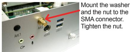
12. Have an external antenna. Screw and tightly fasten the antenna to the SMA connector.
