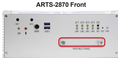
2. Loosen the screws and pull out the bracket.
