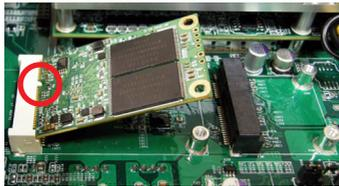
The module's key notch should meet the connector's break.
