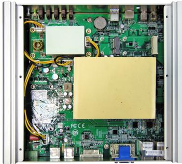
2. Find the two **PCI Express Mini-card** sockets for a WiFi module. The socket has a break among the connector.
