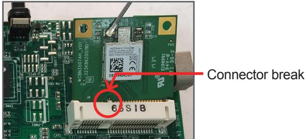
6. Press the module down and fix the module in place using one screw.
