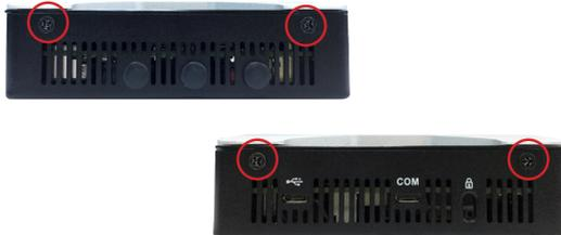
3. Fasten the 3 screws on the rear panel of the chassis.
