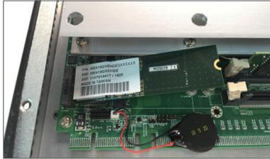
3. Press the module down and fix the module in place using one screw.
