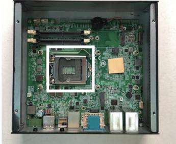
The processor socket comes with a lever to secure the processor. Please refer to the pictures step by step as below and note that the cover of the socket must always be installed during transportation to avoid damage to the socket.
