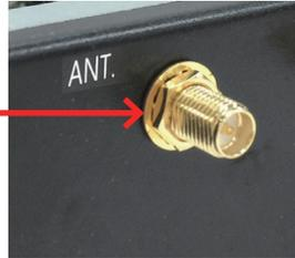
7. Have the external antenna(s). Screw and tightly fasten the antenna(s) to the SMA connector(s).
