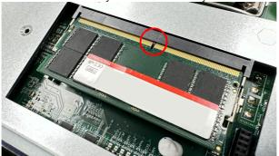
4. Pluh the module into place. Once the memory module is fully inserted into the socket, press down on the top edge of the device to latch it into place.
