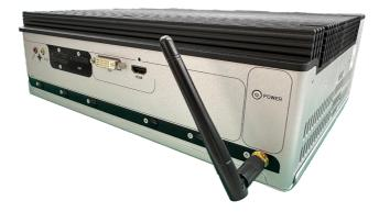
12. Have the external antenna(s). Screw and tightly fasten the antenna(s) to the SMA connector.
