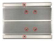
2. Loosen and remove the 2 screws on the front and rear panels respectively as shown below.
