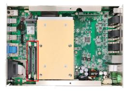
The SO-DIMM sockets are vertical type, and each socket has two latches for fixing the memory modules. The memory module can only be installed by one direction due to the notch.
