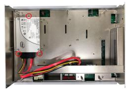
5. Connect the SATA signal cable and power cable.
