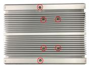
2. Loosen and remove the 4 screws on the front and rear panels respectively as shown below.
