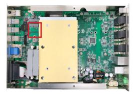
3. Prepare the Wi-Fi module kit. The module is a **M.2 E-Key** socket form factor, with two U.FL connectors, one is "MAIN", and the other is "AUX".
