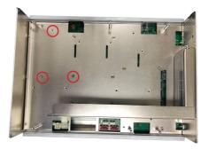
3. Attached the SATA cable to the HDD/SSD storage device. Slide the HDD/SSD storage device into the bracket and fix the storage device in place by fastening the 2 screws on both sides of the bracket.
