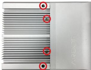
2. Loosen and remove the 2 screws on the front and rear panels respectively as shown below.
