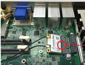
The module's key notch should meet the connector's break.
