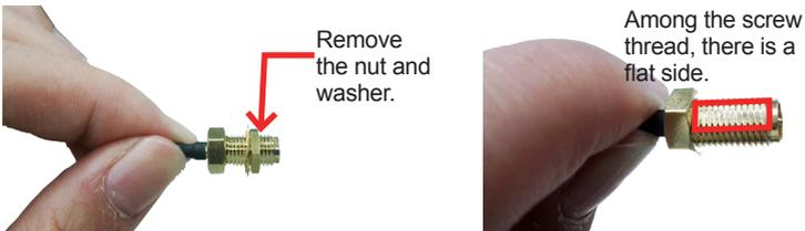
8. Pull the SMA connector through the above mentioned antenna hole. Note to meet the aforesaid flattened side with the antenna hole's flat side.
