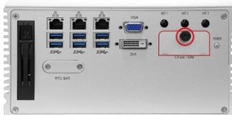
2. Once the screw is removed, open the door. The CFast slot then comes to view.
