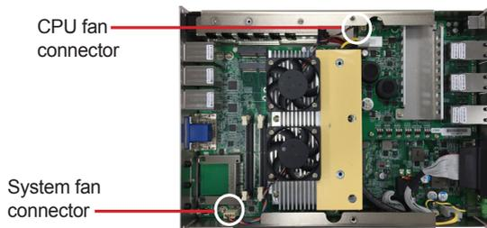
**Caution:** Make sure the fan cables are properly routed. DO NOT route the cables over the heat sink.
