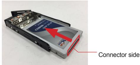
4. Fix the storage device in place by fastening the 2 screws on both sides of the tray .
