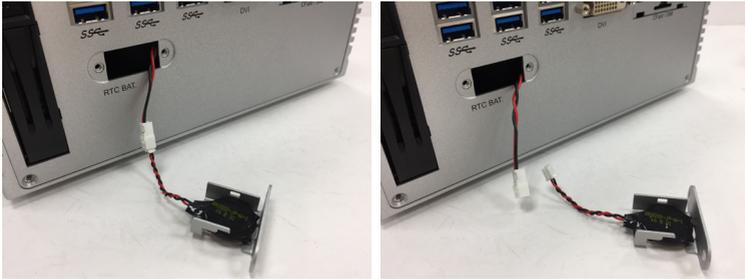
3. Using a non-metallic tool, pry up the RTC battery from the adhesive that secures it to bracket.
