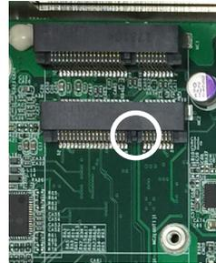
The module's key notch should meet the connector's break.
