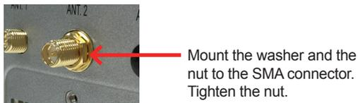
10. Have the external antenna(s). Screw and tightly fasten the antenna(s) to the SMA connector.
