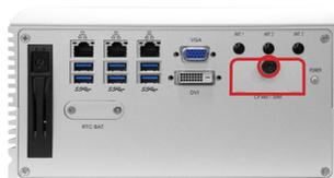
Note: Be sure to turn off the computer before installing or uninstalling the CF card if the OS is installed on the card.
