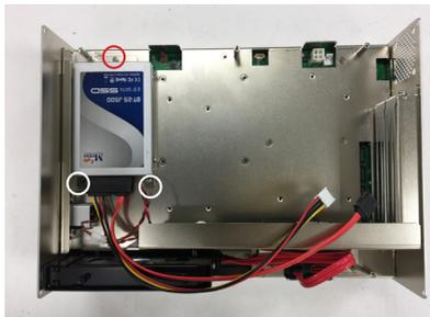
5. Connect the SATA signal cable and power cable.
