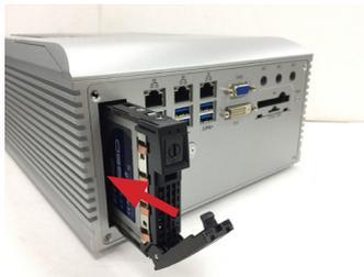
6. Press the eject button first to further slide in the tray. (Do not press the lever directly.) When the lever returns a little bit, press the lever to completely slide the tray back into the drive bay.
