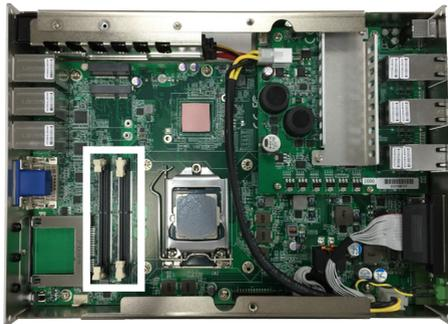
The SO-DIMM sockets are vertical type, and each socket has two latches for fixing the memory modules. The memory module can only be installed by one direction due to the notch.
