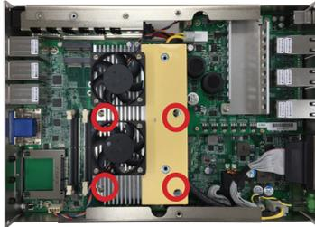
8. Restore the top cover to the computer by fastening the 4 screws as shown below. Note that the 2 screws in the middle are used to secure the top cover to the heat sink. Make sure they are tightened to ensure the heat dissipation.
