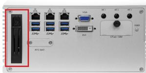
1. The outside accessible HDD/SSD tray comes with a lock. To eject the tray, use a flat head screwdriver to unlock the tray.
