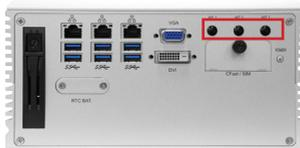
7. From the SMA end of the RF antenna, remove the washer and the nut. Save the washer and nut for later use. Note that the SMA connector is in the form of a threaded bolt, with one flat side.
