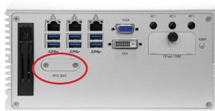
2. Pull out the RTC battery and disconnect the battery cable from its connector on the system board.
