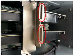
Use a cross-head screwdriver to tighten screws on the graphic card bracket.
