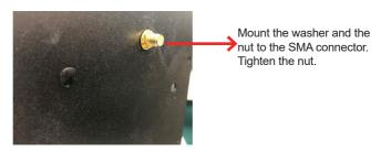
12. Have the external antenna(s). Screw and tightly fasten the antenna(s) to the SMA connector.
