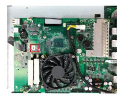
3. Slide the SIM card holder cover towards the OPEN edge and then lift the cover to open it.
