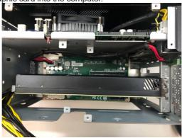
3. Use a cross head screwdriver to tighten the screws to secure the graphic card.
