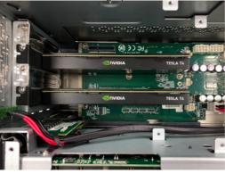
3. Use a cross-head screwdriver to tighten the screws to secure the graphic card holder.
