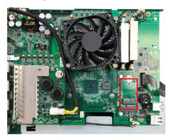
3. Prepare the Wi-Fi module kit. The module is a **M.2 E-Key** socket form factor, with two U.FL connectors, one is "MAIN", and the other is "AUX".
