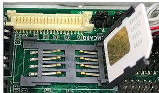
3. Close the SIM card holder door and slide the door to the LOCK edge to lock into place.
