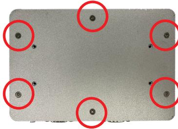
2. Remove the bottom cover completely from the computer.
