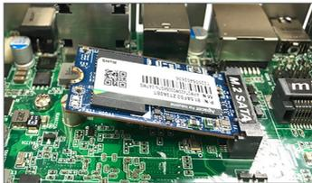
2. Press the module down and fix the module in place using one screw.
