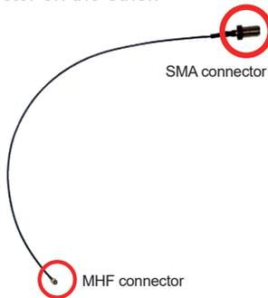
3. Connect the RF antenna's MHF connector to the Wi-Fi module's main connector marked 0.
