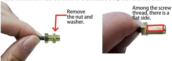
9. Pull the SMA connector through the above mentioned antenna hole. Note to meet the aforesaid flattened side with the antenna hole's flat side.
