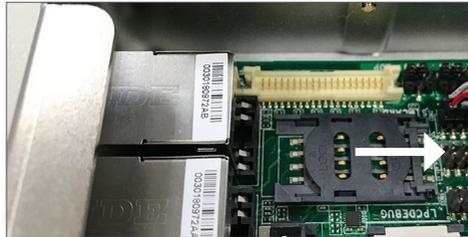
2. Insert the SIM card into the card holder as shown below.
