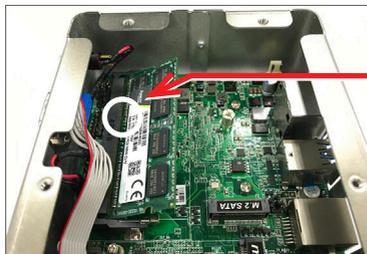
Align the memory module's key notch at the SO-DIMM slot connector's break.
