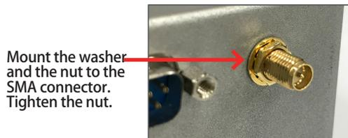
11. Have the external antenna(s). Screw and tightly fasten the antenna(s) to the SMA connector(s).
