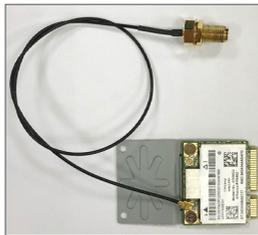
5. Plug the Wi-Fi module to the socket's connector by a slanted angle. Fully plug the module, and note the notch on the wireless module should meet the break of the connector.
