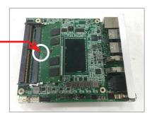
3. Press down the memory module until it is auto-locked in place.
