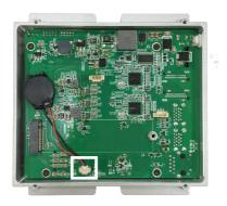
3. Using a non-metallic tool, pry up the RTC battery from the adhesive that secures the battery.
