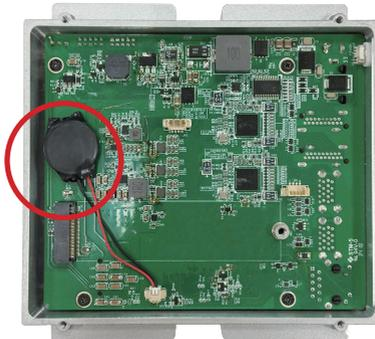
4. With the adhesive side down, place the new RTC battery into position on the system board.
