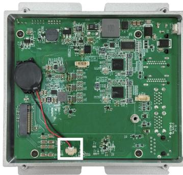
3. Using a non-metallic tool, pry up the RTC battery from the adhesive that secures the battery.
