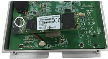
3. Using the screw coming with the SSD module kit, fix the SSD module in plac
