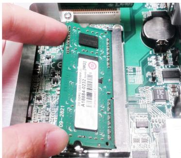
5. Press down the memory module until it gets auto-locked in place.
