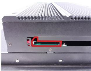
3. Insert a CFast card to the slot. Fully insert the CFast and push-lock the card in place.
