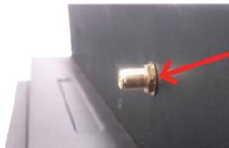
Mount the washer and the nut to the SMA connector. Tighten the nut.
