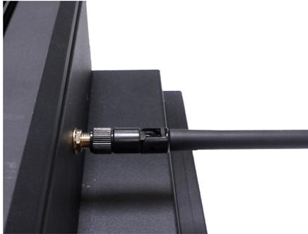
14. Swivel the antenna to an angle of best signals.
