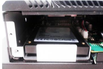
Fully slide the storage bracket and the storage device until they cannot be slid any more.
