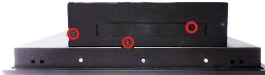
2. Remove the three screws from the left panel of the computer as the illustration above shows.
