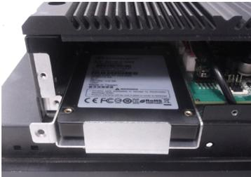
Slide the storage and the bracket back into the computer.
