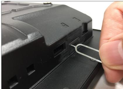
3. After ejecting the SIM card tray, place your SIM card into the tray. Note that there is notch in one corner to ensure the SIM card is placed correctly.
