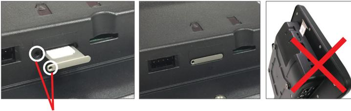
Make sure to align the hole on the tray with the hole in the device.
