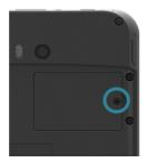
Figure 2-1 Screw off and remove the cover.
