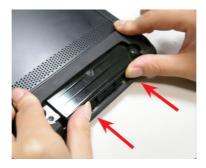
6. Replace the battery cover and secure the retaining screws with a coin.
