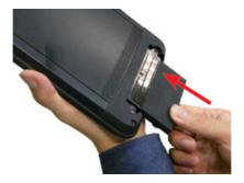
3. To restore the protective lid, make sure the lid is oriented as shown in the photo to the right.
