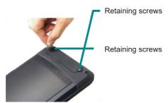
2. Remove the battery cover using the notch located on the bottom edge.
