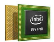
So the quad-core Celeron J1900 processor powering ARBOR's ASLAN Industrial Panel PC packs far more of a punch than earlier chips in fanless packages, even though its thermal design power is just 10 watts, less than that of even ultra-low voltage mobile Intel Core processors.
