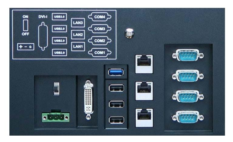
While the optimal design and configuration of Industry 4.0 hardware componentry may not have fully emerged just yet, ARBOR is likely on the right track by equipping ASLAN panels with three independent RJ45 LAN interfaces to
