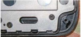
The interior of the Gladius 10 leave a good impression. It is a well conceived and executed design that's very structurally stable. The sole concerns we have are the long o-rings that can easily get damaged, and the snap-together design of the housing and the battery compartment cover.
