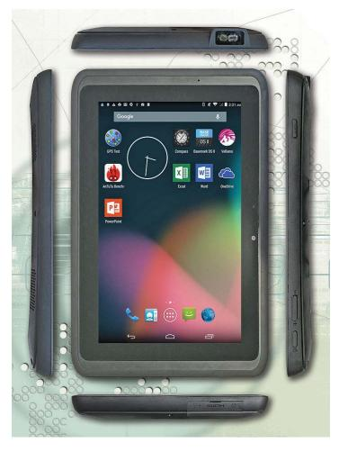
Going around the Gladius 10 reveals the necessary minimum of controls and ports. This is a well-sealed device, and that means the fewer openings that must be protected against immersion the better.
