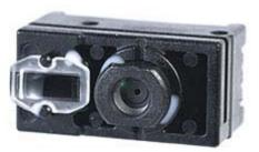
Below you can see close-ups of some of the interesting details of the ARBOR Gladius 10. On the left is one of the nicely sized speakers mounted inside its own protective metal seat. It'll never come loose by accident. In the center is another look at the tablet's industrial-grade Opticon barcode reader. On the right are the SIM and micro SD card slots.
