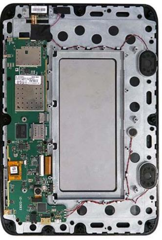
The top half of the tablet consists of the unit's exceptionally sturdy magnesium frame that has the LCD assembly mounted on one side, and the tablet's electronics on the other. Compared to virtually all x86 Windows tablet designs, the Gladius is amazingly sparse and clean inside. The slender system board measures 8-1/2 x 2 inches and looks as neat and simple as something from Apple. No busy layout here, and no complex stacked daughterboards and modules.
