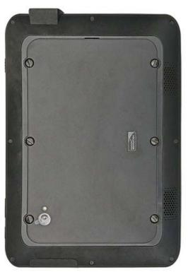
The removable plastic plate that provides access to the battery and card slots is secured with six large screws that can be opened with a flat screw driver, a coin, or even a fingernail. The design is such that the screws won't fall out, which is much appreciated. Carefully unsnap the cover to see the flat (only 8mm thick) 3.8 Volt 9,300mAH 35 watt-hour battery that neatly fits into a compartment of the metal frame.
