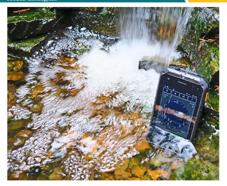
The impressive strength provided by the GT-500's internal magnesium frame suggests a high degree of toughness and ability to withstand accidents and abuse. And the device does feel absolutely rock-solid. External ports all have tight-fitting protective rubber plugs with their own replaceable o-ring seals.
