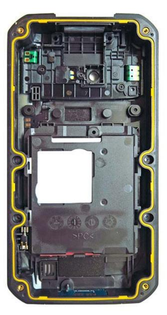
The poly-carbonate housing has fused black rubber overmoldings that make the device grippier and easier to hold, and they also provide extra protection. Sealing between the two halves of the GT-500 housing is via an elaborate tongue-and-groove design that uses a precision-cut bright yellow replaceable seal for best possible protection.
