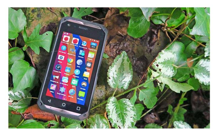
IP67 sealing means the GT-500 is totally dustproof and can even handle total immersion in water. It can survive 5-foot drops thanks to its tough internal magnesium frame and substantial external protection. Despite its solid build, the GT-500 remains compact, pocketable, and suitable for one-handed operation.
