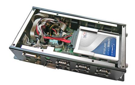
What the ARES-1231 brings to the table is a full 16 COM ports, and a full set of 16 DI and 16 DO ports. Of the COM ports, they all use standard DB9 connectors, but they come in three different configurations. Eight can be set to be either RS-232 or RS-485, four are DIM switch selectable for RS-232/422/485, and four are PIN-header selectable between RS-232 and RS-485. The digital IO ports use two DB26 connectors with 8DI and 8DO each.
