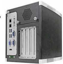
Interconnect Express) is a faster, improved version of PCI, and the ARES-1970-4E can be equipped with up to four X1 single lane cards.
