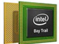
The Celeron N2930 CPU is part of Intel's next-gen "Bay Trail" platform which employs 22nm process technology and has integrated graphics cores of the same HD 4000 architecture and variety as those used in Intel's 3rd generation "Ivy Bridge" processors, albeit with fewer execution units (four instead of several times that number) and lower clock speeds. The N2930 is also the same chip ARBOR used in its Gladius G0975 rugged tablet ([see our review of the G0975](#)).
